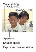
Aperture—also referred to as f-stop, controls the size of the lens opening, which determines the depth of field. Larger aperture settings keep both foreground and background sharp, good for landscapes and well-lit conditions. Smaller aperture settings make the foreground sharp and background blurry, good for portraits and low-light conditions. The highest and lowest aperture settings may be affected when using optical zoom.
