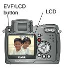
Your camera is equipped with an electronic viewfinder (EVF). The EVF, like the LCD screen, displays exactly what the camera captures.
